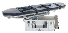
Spectrum Aeromed's extremely versatile 2800 Series is lightweight, compact and fits smaller aircraft, yet has critical care capabilities for larger aircraft as well. This system can be installed in single- or multiple-patient configurations depending on cabin space.
