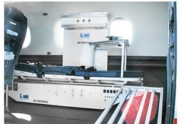
Stretcher and Base Install
