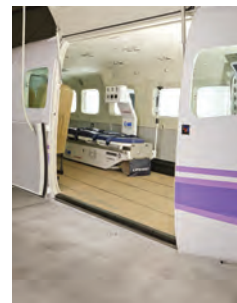
2800 series module installed in 208B
