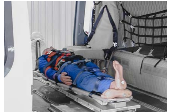
Pivot base installed longitudinally and laterally in the aircraft.
